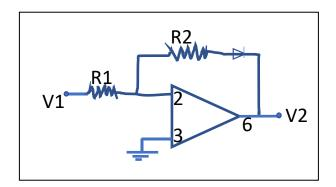
3) In the adjacent diode circuit, R1=20k $\Omega$ , R2=10k $\Omega$ , Vin(t)=12 cos(t) Volts, and the forward voltage across diode is 0.65 V.
